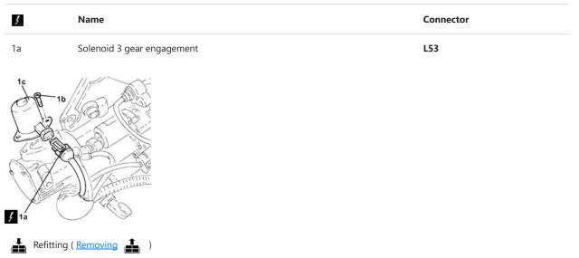
Fit the gear selection solenoid in its seating and tighten the fixing bolts.
